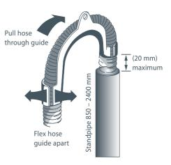
Fig.2 Fitting the drain hose guide
